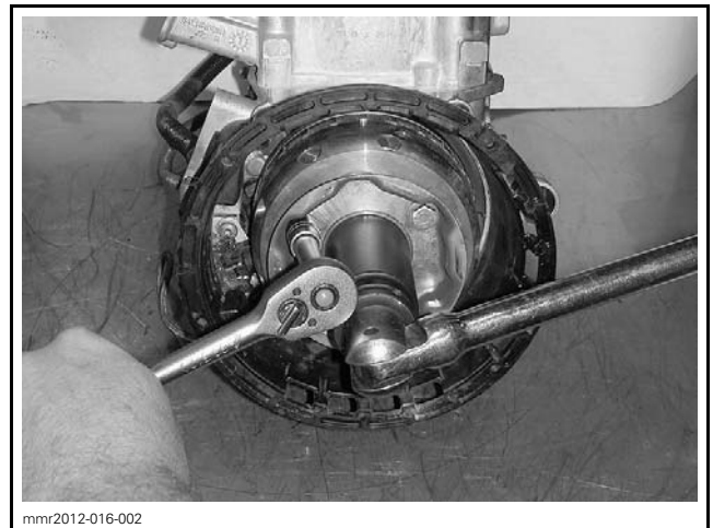
mmr2012-016-002 TYPICAL - STARTING PULLEY SCREWS REMOVAL
