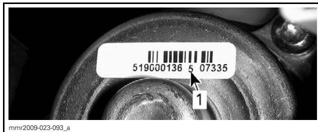
BACK OF OIL INJECTION PUMP
