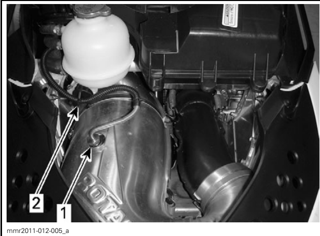
1. Tuned pipe temperature sensor 2. Coolant tank support
