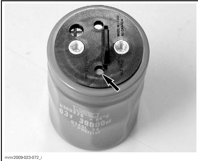
INSPECTION HOLE (SHIELD IS INTACT)
