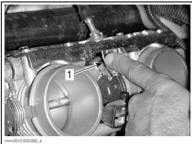
THROTTLE CABLE FREE PLAY 1. Cable slightly loose here
