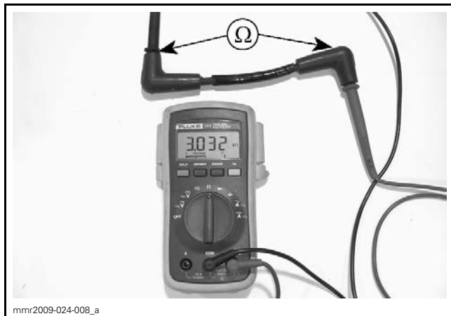
SPARK PLUG CABLE RESISTANCE TEST
