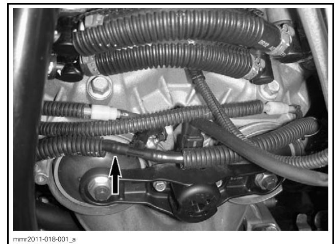
INLET HOSE AT T-FITTING
