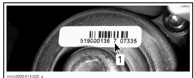
BACK OF OIL INJECTION PUMP
