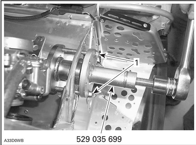
1. Screws replacing bearing support screws
