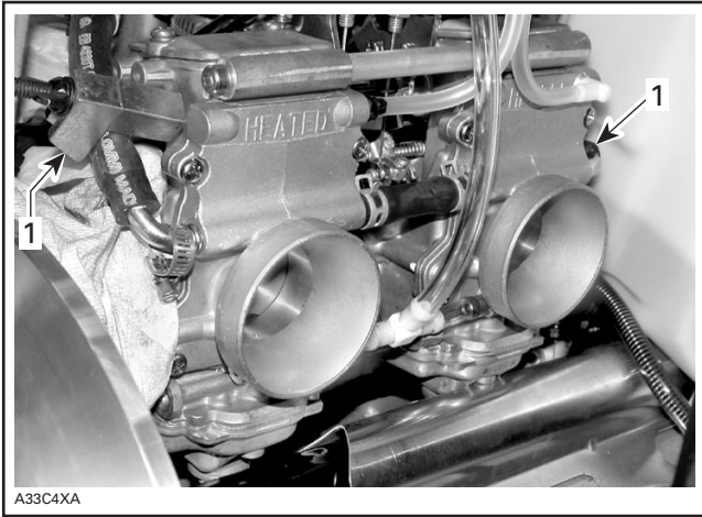
1. Install hose pinchers
