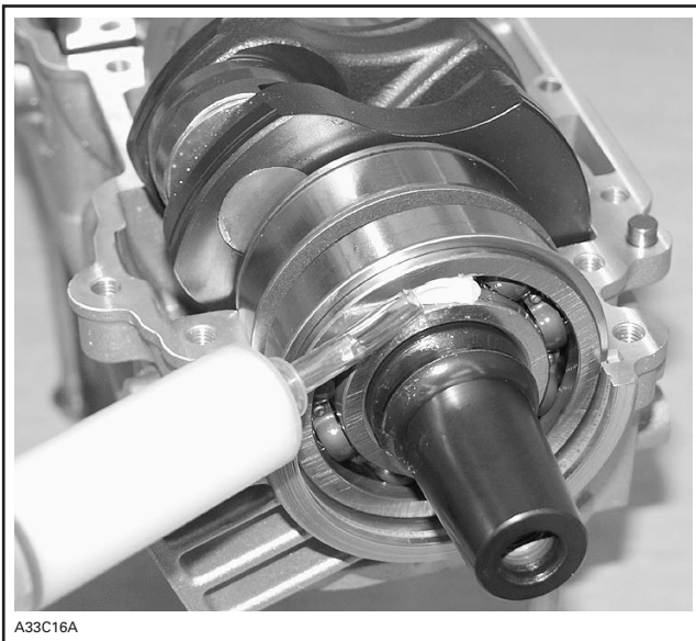
BALLS COATED WITH A SEAM OF GREASE
