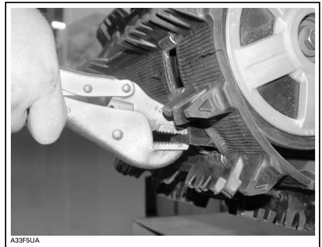
TYPICAL — PULL ON SLIDER SHOE TO REMOVE
