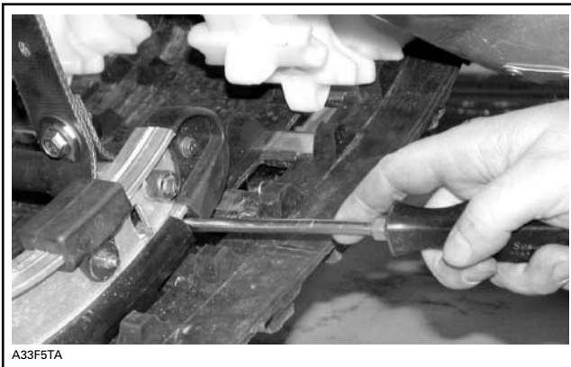
TYPICAL — PUSH ON SLIDER SHOE
