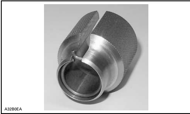
CIRCLIP READY TO BE INSTALLED ON PISTON
