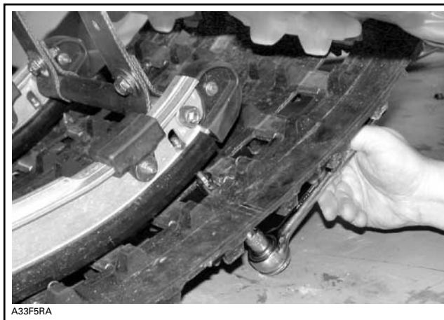
TYPICAL — REMOVE NUT AND SCREW
