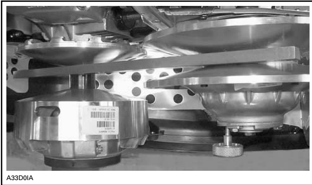
TYPICAL — ALIGNMENT BAR IN PULLEYS
