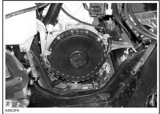
RH SIDE — MAGNETO HARNESS ROUTING
