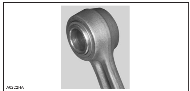
TYPICAL — CAGELESS BEARING AND SLEEVE INSTALLED
