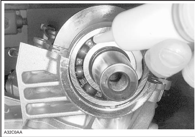
BALLS COATED WITH A SEAM OF GREASE
