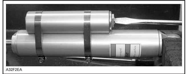
DISCHARGING GAS PRESSURE
