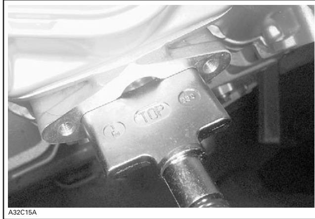
RAVE VALVE PARTIALLY REMOVED
