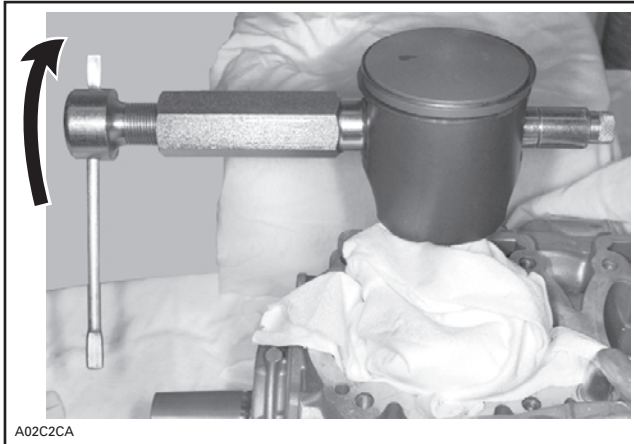
TYPICAL — PISTON PIN EXTRACTION
