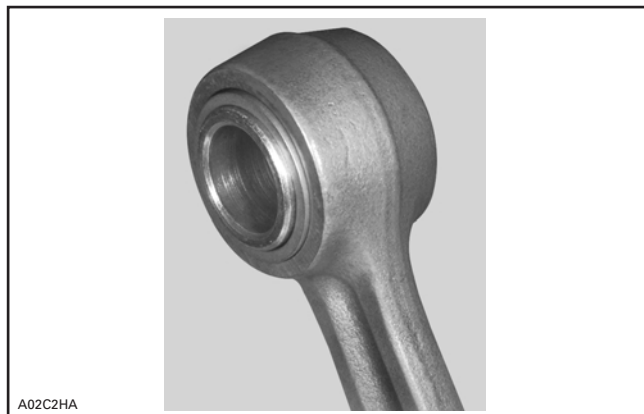
TYPICAL — CAGELESS BEARING AND SLEEVE INSTALLED
