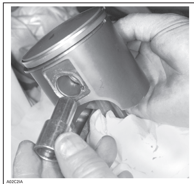
TYPICAL — SHOULDERED SLEEVE INSTALLATION
