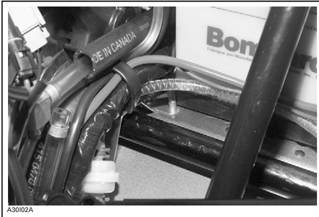
VENT TUBE PROPERLY CONNECTED
