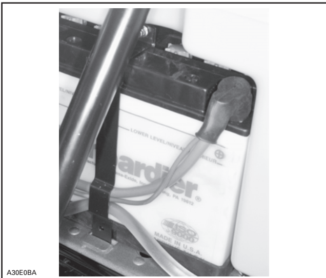
RED POSITIVE (+) BATTERY CABLE AND WIRE POSITIONING
