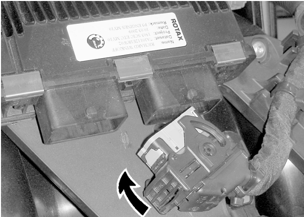
CONNECTOR LOCKING CAM IN RELEASE POSITION
