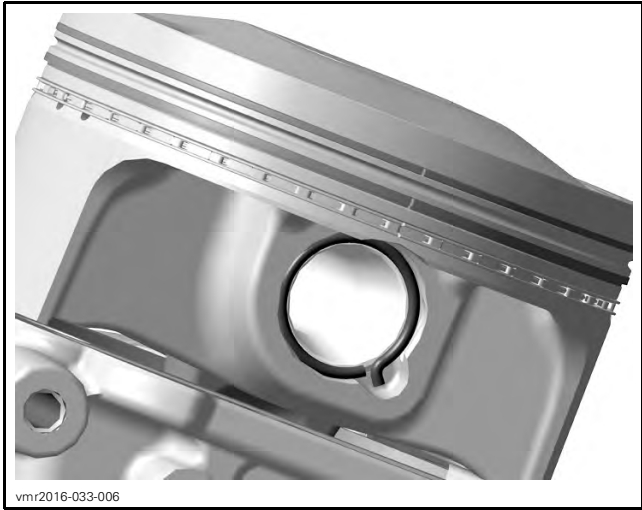
CORRECT POSITION OF THE PISTON CIRCLIP
