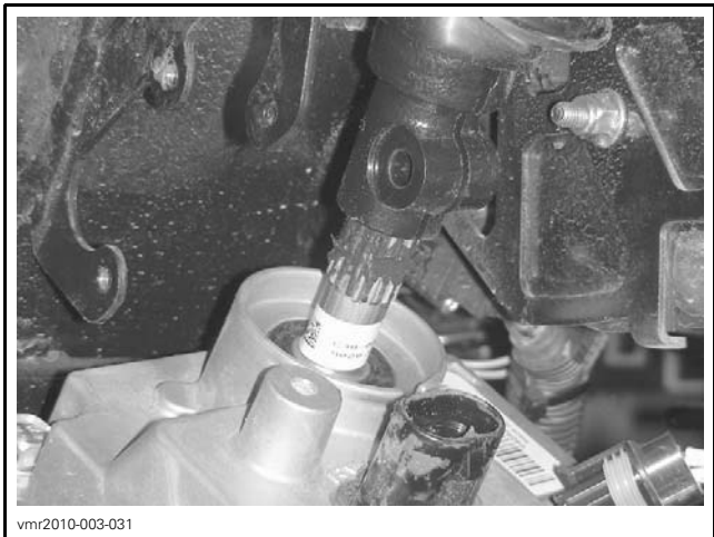
vmr2010-003-031 TYPICAL - STEERING COLUMN INDEXED TO DPS SHAFT SPLINES
