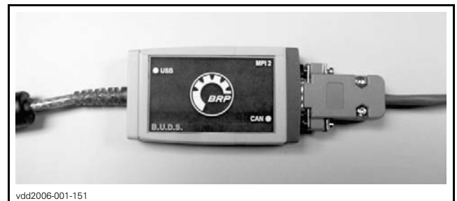
DIAGNOSTIC CABLE CONNECTED TO MPI-2 INTERFACE CARD
