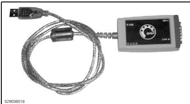
MPI-2 INTERFACE CARD CONNECTED TO USB PORT
