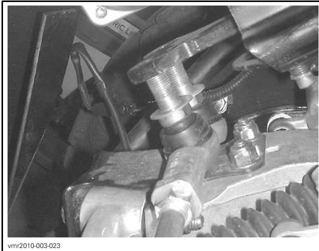
TYPICAL - TIE ROD ENDS (HARDWARE REMOVED)
