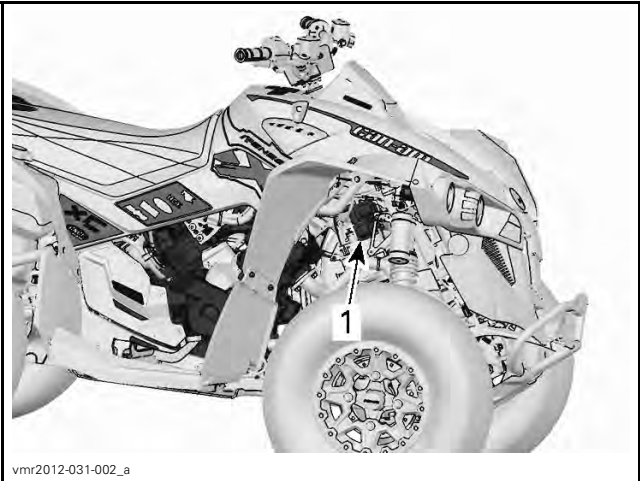
TYPICAL 1. Ignition coil location
