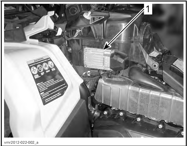
LH PANEL REMOVED 1. ECM location
