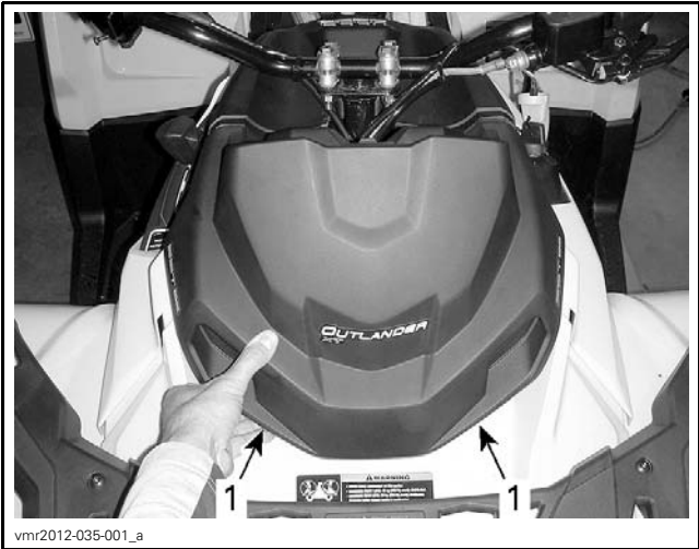
OUTLANDER GAUGE SUPPORT REMOVAL 1. Push in and lift up here (both sides)
