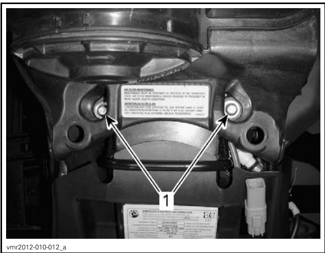
vmr2012-010-012_a SCREWS LOCATED NEAR SEAT ANCHORAGE 1. Air filter housing retaining screws
