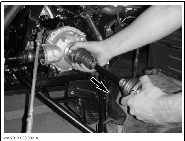
PULL DRIVE SHAFT
