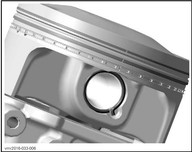
CORRECT POSITION OF THE PISTON CIRCLIP
