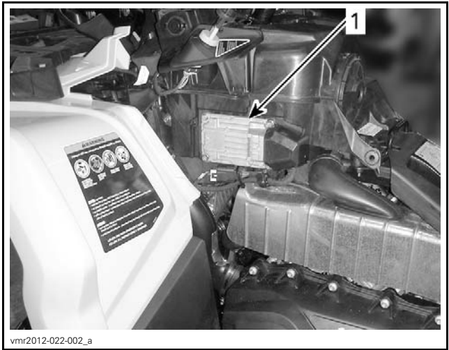
LH PANEL REMOVED 1. ECM location
