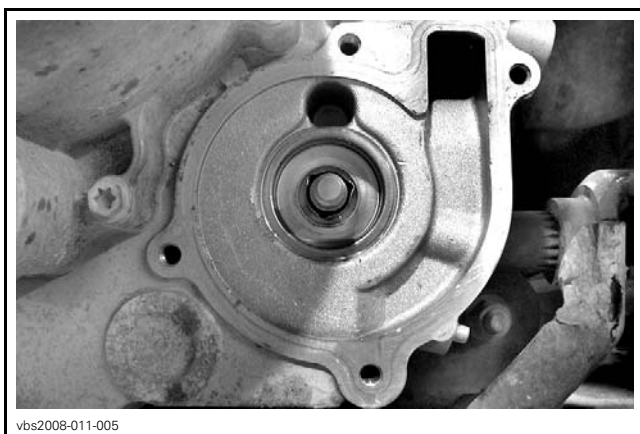
TYPICAL - INNER PART OF ROTARY SEAL REMOVED
