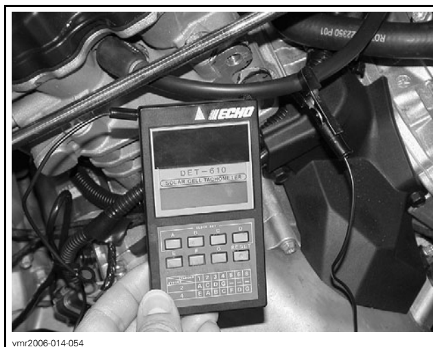
vmr2006-014-054 VERIFYING ENGINE RPM USING A DIGITAL INDUCTION TACHOMETER
