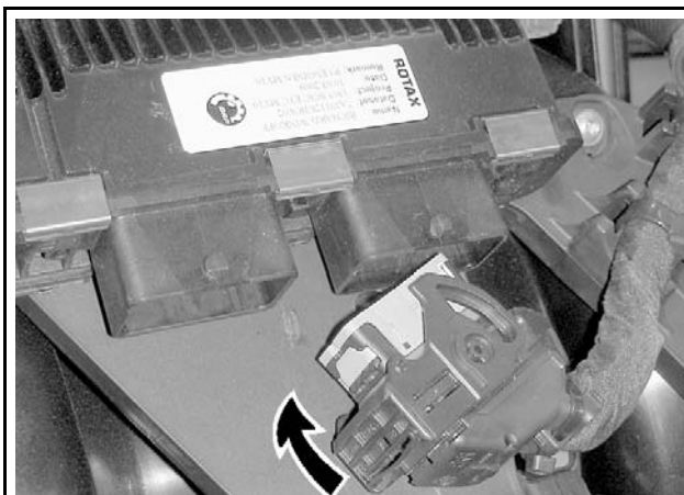
CONNECTOR LOCKING CAM IN RELEASE POSITION
