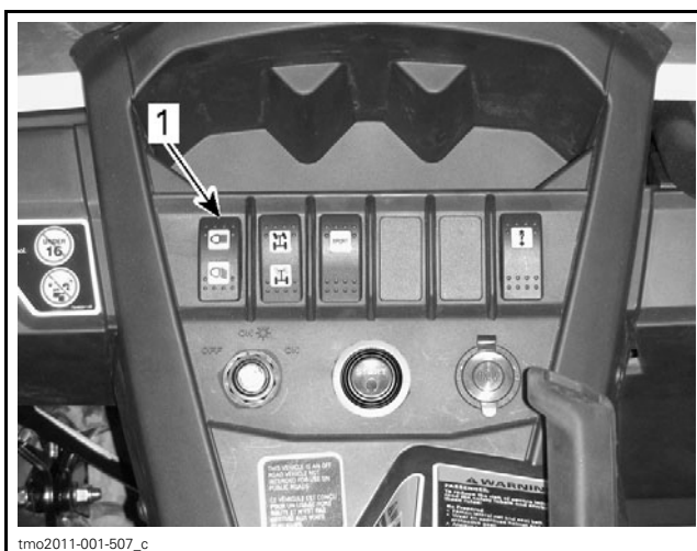
1. Low/High beam headlight switch to toggle quickly
