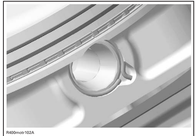
CORRECT POSITION OF THE PISTON CIRCLIP
