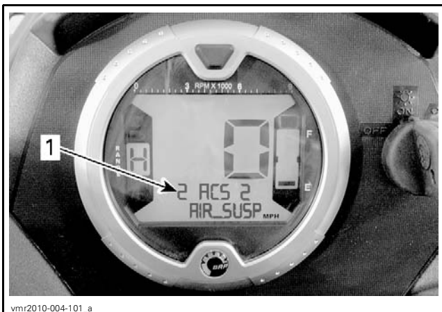
1. Actual setting (pressure transducer reading)
