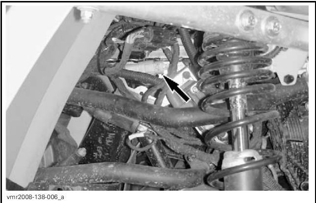
STATOR CONNECTOR, INNER FENDER PANEL REMOVED
