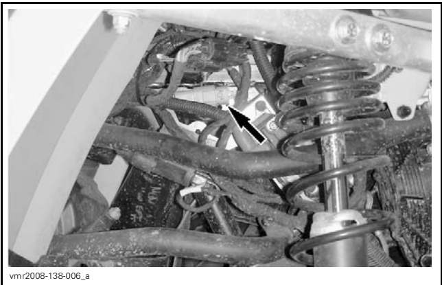
STATOR CONNECTOR, INNER FENDER PANEL REMOVED
