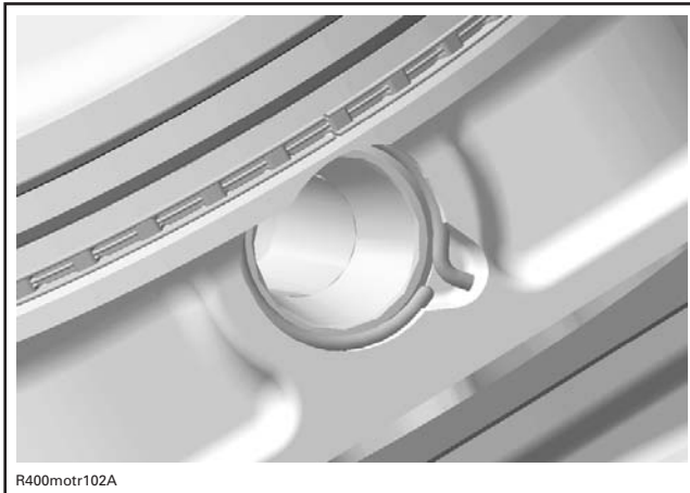
CORRECT POSITION OF THE PISTON CIRCLIP
