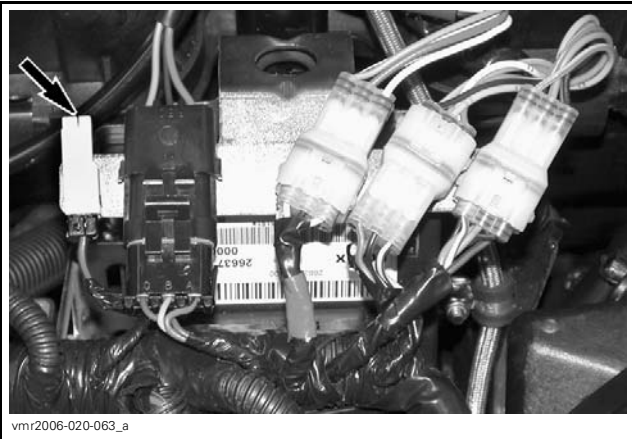
TYPICAL – AUXILIARY POWER CONNECTOR
