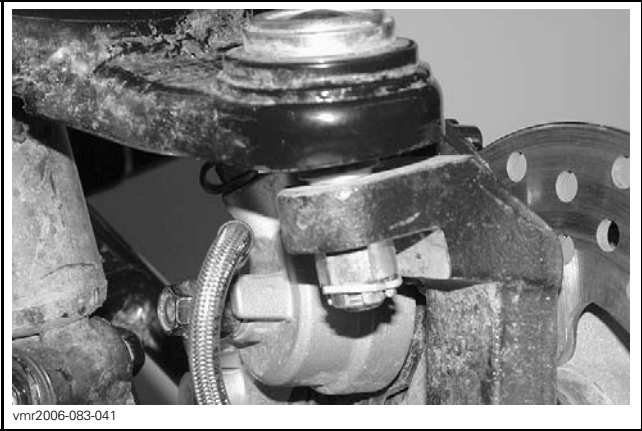
Remove bolts retaining A-arm to frame.
