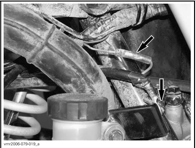
BATTERY AND IGNITION MODULE GROUNDS (CLOSE TO REAR BRAKE MASTER CYLINDER)
