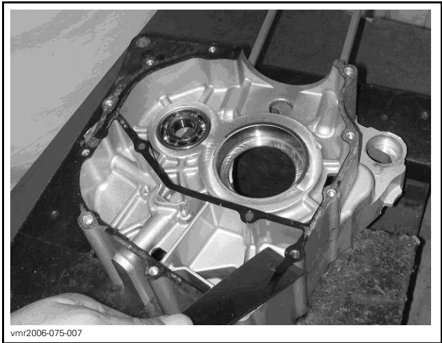
Remove gasket and dowel pins. Scrape gasket residues off the crankcase contact surface.
