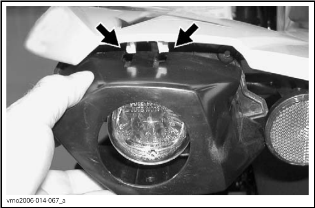
RELEASE HOUSING FROM REAR FENDER
