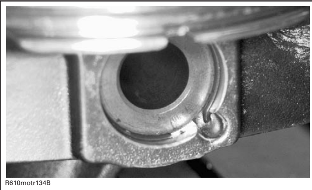
CORRECT POSITION OF THE PISTON CIRCLIP
