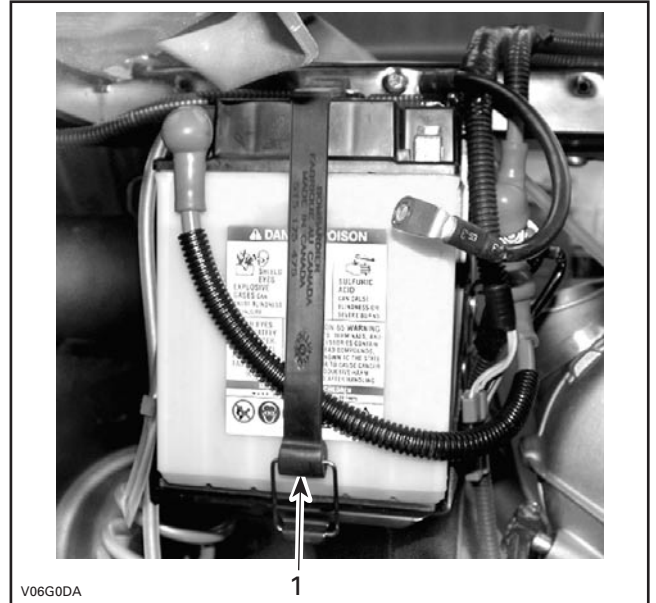
1. Cable between battery and strap
