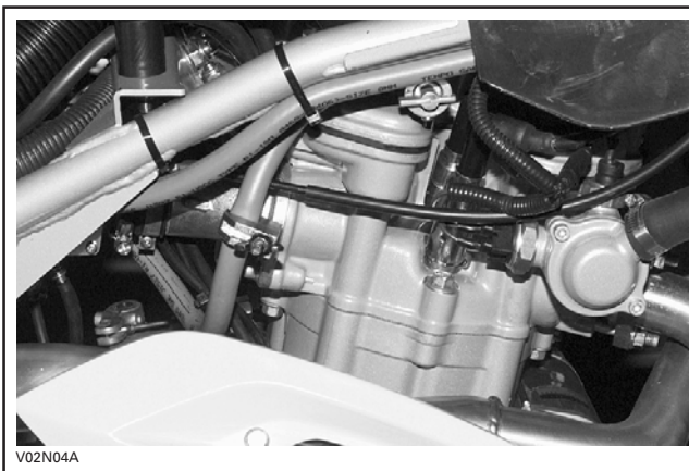
HOSE PINCHER INSTALLED ON FUEL PUMP OUTLET
