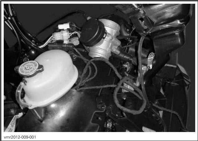
TYPICAL - THROTTLE BODY ATTACHED ON FRAME
