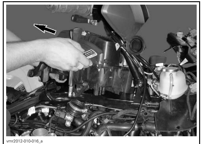
vmr2012-010-016_a AIR FILTER HOUSING REMOVAL
