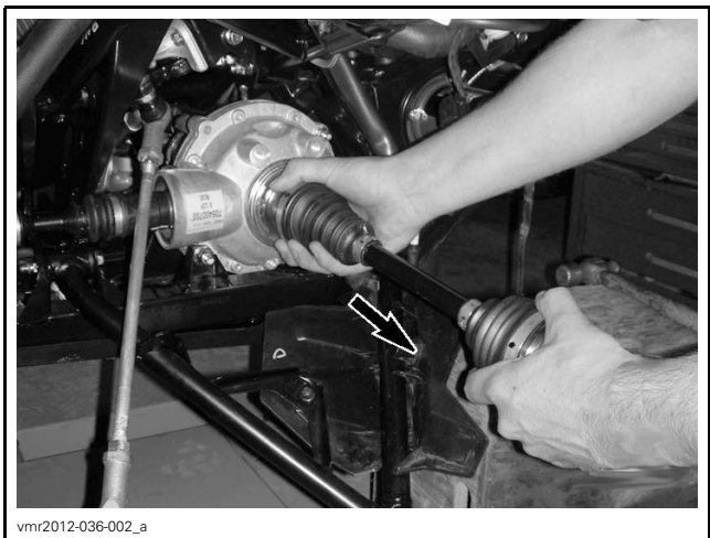
PULL DRIVE SHAFT
