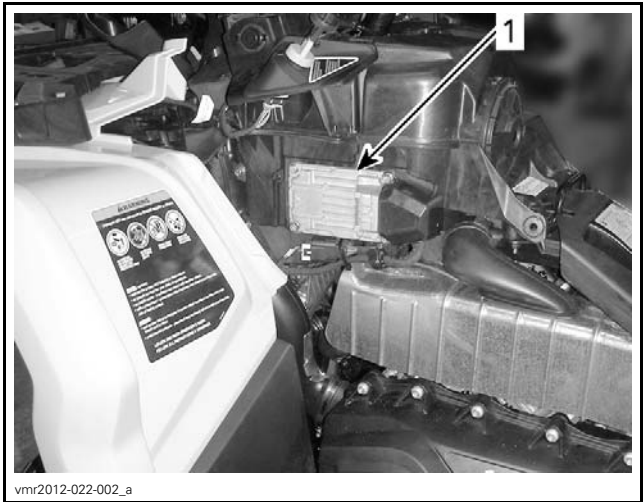
LH PANEL REMOVED 1. ECM location
