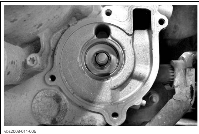
TYPICAL - INNER PART OF ROTARY SEAL REMOVED
