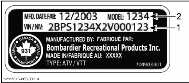
TYPICAL — VEHICLE SERIAL NUMBER DECAL ON RH SIDE OF FRAME 1. VIN (Vehicle Identification Number) 2. Vehicle manufacturing date and model number
