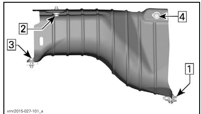
REAR HEAT SHIELD TIGHTENING SEQUENCE
