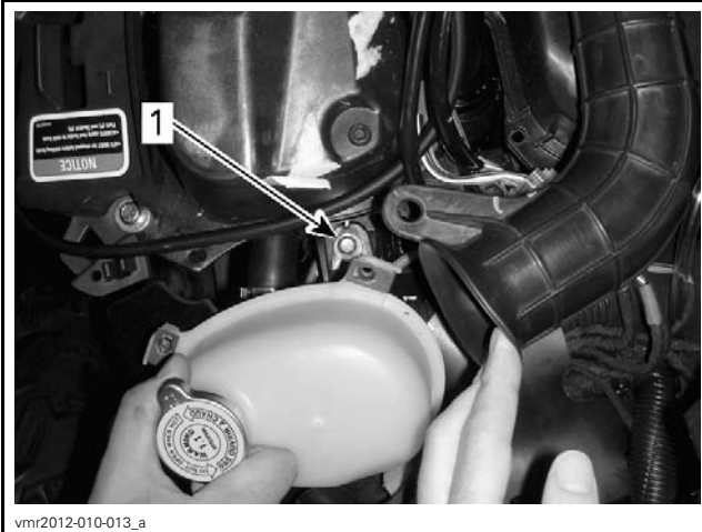
vmr2012-010-013_a SCREW LOCATED UNDER COOLANT TANK 1. Air filter housing retaining screw
