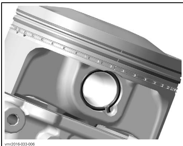
CORRECT POSITION OF THE PISTON CIRCLIP
