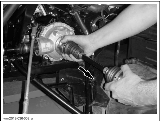
PULL DRIVE SHAFT
