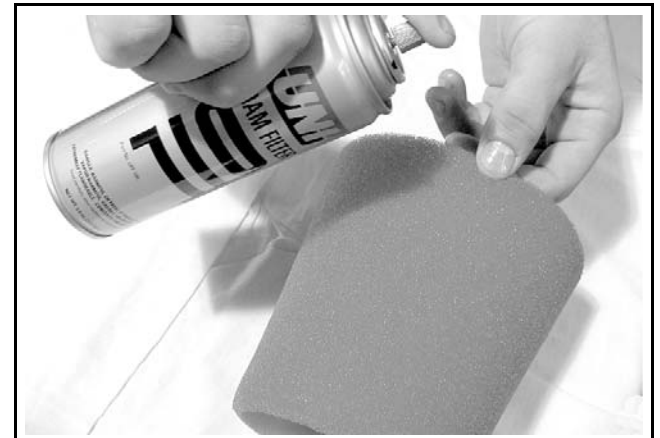
TYPICAL - OIL THE FOAM FILTER
