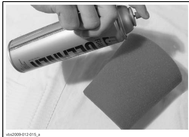
TYPICAL - SPRAY THE FOAM FILTER
