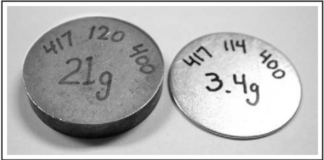
Photo shows the 2 different types of weight used in BOMBARDIER LITE clutches.
